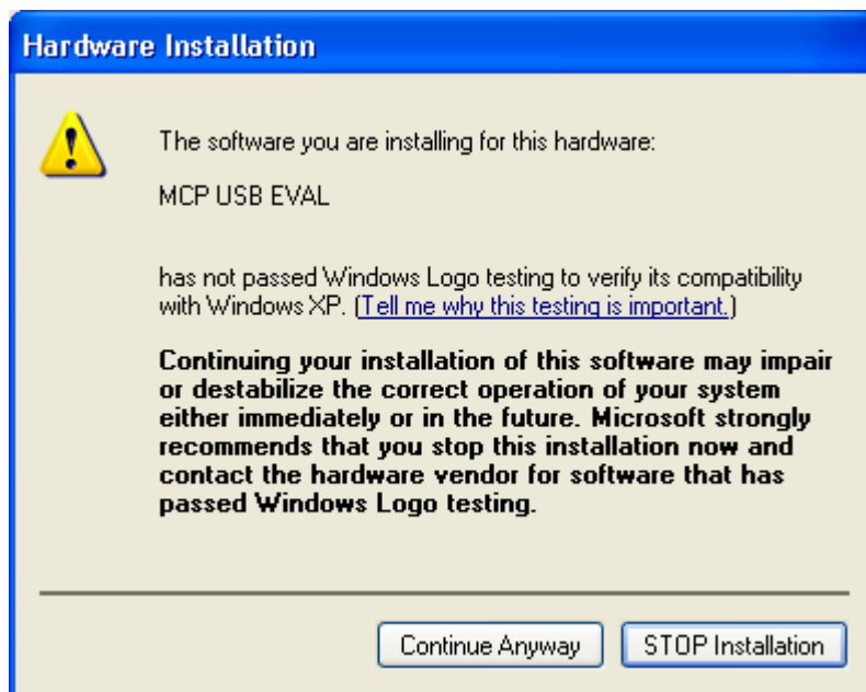
Figure 8. USB Driver Hardware Installation (Click on Continue Anyway)
