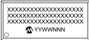
28-Lead SOIC (7.50 mm)
