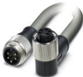
Bus system cable, DeviceNet, 5-position, PVC, Gray RAL 7001, Plug straight 7/8"-16UNF, on Socket angled 7/8"-16UNF, Cable length: 0.3 m
