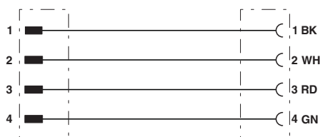
Contact assignment of 7/8" plugs/sockets
