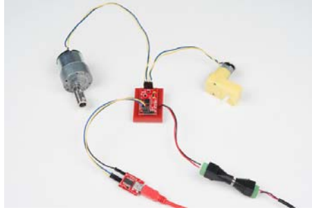
A SCMD ready to drive motors from UART command.
