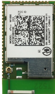
Figure 2: xPico W1003 (XPC W1003) Embedded Device Server
