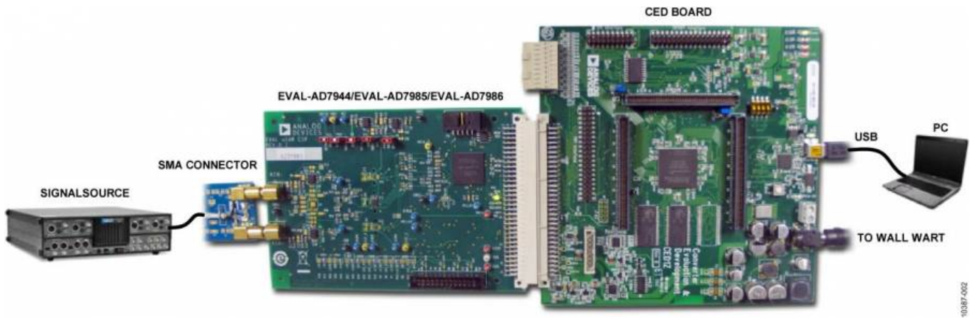
Figure 2. Hardware Configuration—Setting up the Evaluation Board
