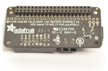
If you're using a 64x64 RGB matrix and a bonnet, use your soldering iron to melt a blob of solder on the bottom solder jumper so the middle pad is 'shorted' to 8
