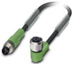
Sensor/actuator cable, 3-position, Variable cable type, Plug straight M8, on Socket angled M12 SPEEDCON, A-coded, cable length: Free input (0.2 ... 40.0 m)
