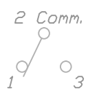
CIRCUIT: SPDT CONTACT CONFIGURATION
