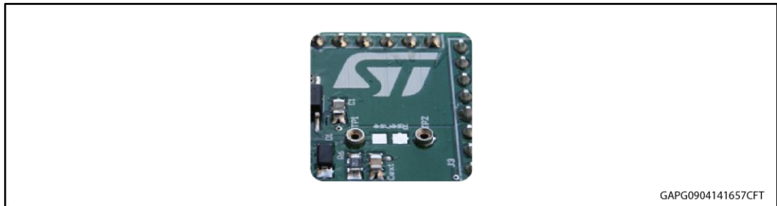
Figure 4: Mounting through-hole sense resistor
