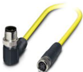
Sensor/Actuator cable, 4-position, PVC, yellow, shielded, Plug angled M12 SPEEDCON, A-coded, on Socket straight M8, Cable length: 1.5 m
