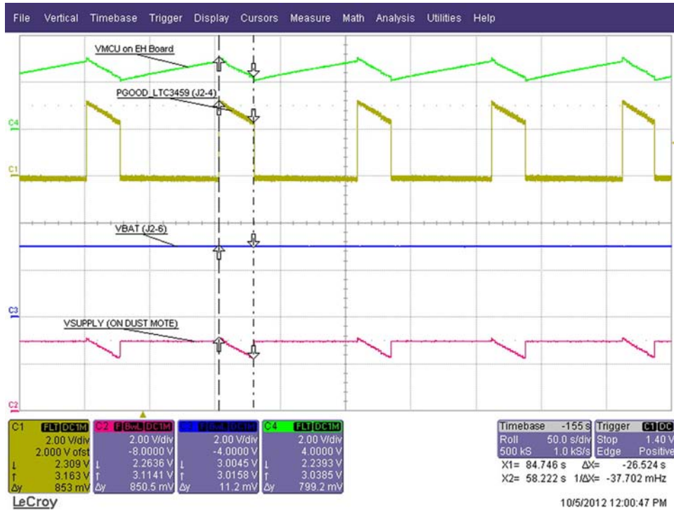
Figure 14: DC2042A LTC3459 Operation at 100 lux with Indy4100 Solar Panel
