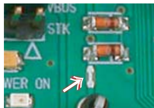
Figure 2-10 . Configuration Pad Location
