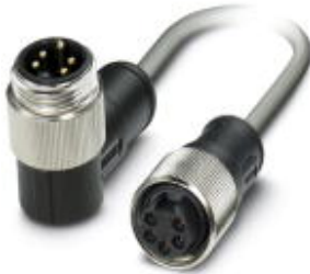
Bus system cable, DeviceNet, 5-position, PUR halogen-free, Gray RAL 7001, Plug angled 7/8"-16UNF, on Socket straight 7/8"-16UNF, Cable length: 20 m
