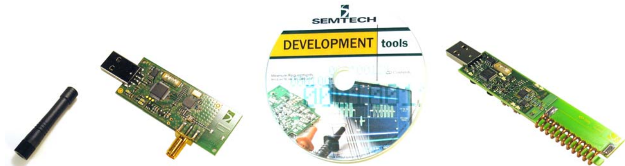
Figure 3: SX1230-12SKA Contents (CR2032 Cell not Shown)
