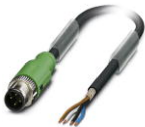
Sensor/actuator cable, 4-position halogen-free, black-gray RAL 7021, shielded, Plug straight M12 SPEEDCON, A-coded, on free cable end, cable length: 10 m
