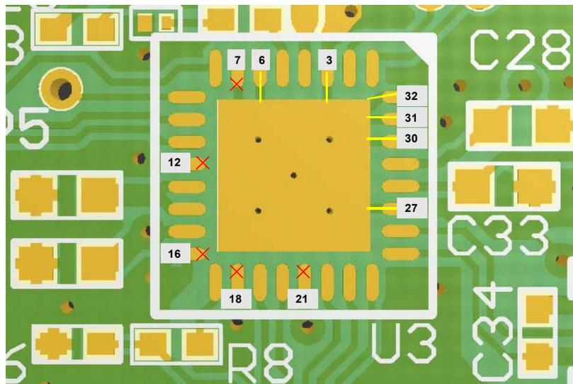
Each ground pin should be connected to the bottom plane with at least one via. Move the vias as close to the IC as possible. It is always desired to integrate the single-pin ground connections into polygon structures after a short distance. Top, bottom, and, on multilayer boards, the inner ground planes, should be tied together with a grid of vias. When ground loops are smaller than one tenth of the wavelength, it is safe to consider this as a solid piece of metal.
