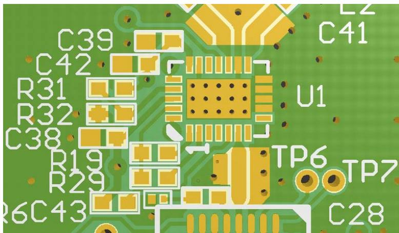
The SE2431L (U1) and associated circuitry follow a standard Skyworks Solutions recommended layout to achieve specified RF performance. The SE2431L requires a central PCB ground pad which is completely relieved of solder resist and has a grid of 15 ground vias [9]. This is essential to achieve good RF performance and adequate thermal conduction, especially in transmit mode. The solder paste mask has limited coverage for assembly purposes.
