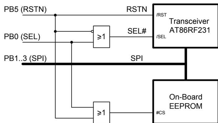
The EEPROM data are written during board production testing. A unique serial number, the MAC address<sup>(1)</sup>, and calibration values are stored. These can be used to optimize system performance.
