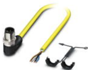
Sensor/Actuator cable, 4-position, PVC, yellow, Plug angled M12 SPEEDCON, A-coded, on free cable end, Cable length: 10 m
