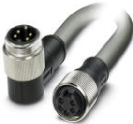
Bus system cable, DeviceNet, 5-position, PVC, Gray RAL 7001, Plug angled 7/8"-16UNF, on Socket straight 7/8"-16UNF, Cable length: 15 m
