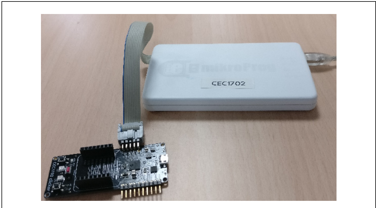
FIGURE B-1: CEC1702 CLICKER BOARD SETUP
