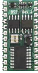
Figure 1-2 BASIC Stamp 2 Microcontroller Module
